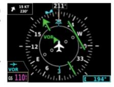
Twisting the selection knob on this page will move the heading bug. Course selection when using VOR/LOC or OBS mode on the GPS can be achieved by pressing the selection knob and twisting to the **Course Tab** and pressing in on the selection knob, you can then twist the knob to select the desired course.
